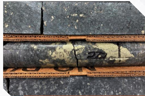
Rip-up clast grades 7.13% Ni, 7.91% Cu over 8 cm sample
